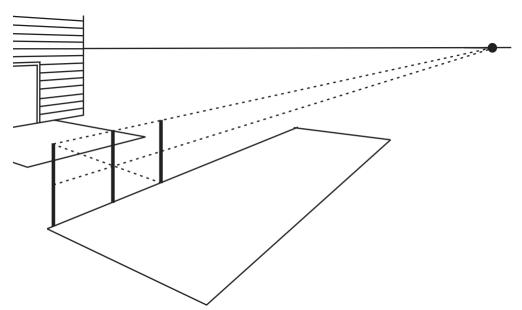
Make a light reference line that goes from the top of the  $1^{st}$  post through the middle of the  $2^{nd}$  post. Where this line touches the ground is where you would place the  $3^{rd}$  post. This technique works for ANYTHING that is lined up and recedes into the distance.
