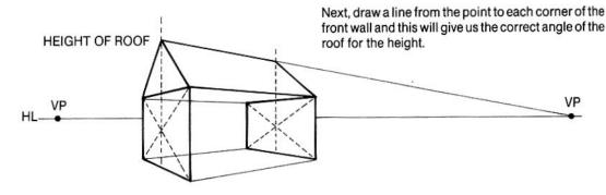
The point where the line for the top of the roof crosses the back vertical center line marks the point and pitch of the roof at the back of the house.
